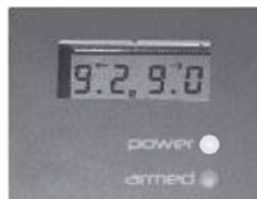
LCD ENERGIZER OUT AND RETURN VOLTAGE DISPLAY
